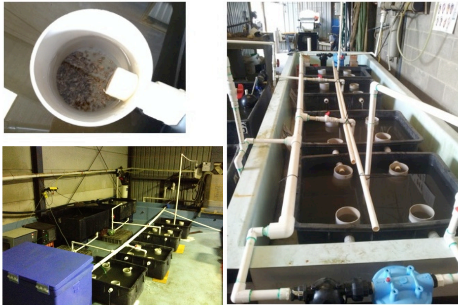
Figure 1. Layout of upwellers in treatment tanks. Top left, detail of upweller. Bottom left, treatment tanks for Trial 1. Right, treatment tanks for Trials 2 to 7; filters are shown in the foreground and at the rear of the main holding tank; the UV unit is wall-mounted.
