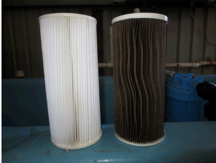
Figure 3. Examples of 5 \mu\text{m} pleated paper filter cartridges. Left, after washing; right, after 1 day in use.
